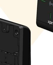
The opening has two breakable squares in the middle. Depending on cabling requirements, one or both squares could be broken. There is also an option for cabling from all four sides as per the wiring.
